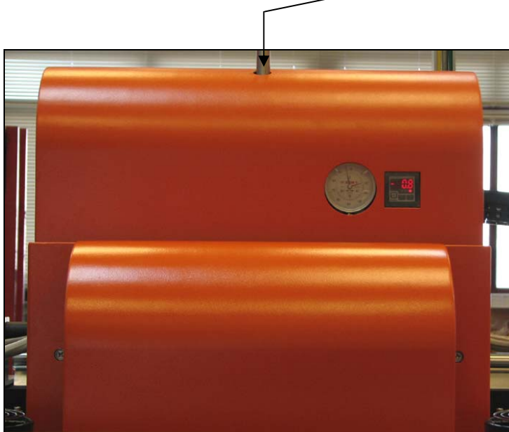
Figure 26: Adjusting the height of the Print Table
